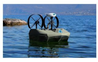
An engineering practice and consultancy specializing in composite materials, **CT2MC** has developed an original solution for taking liquid samples in aquatic environments. Often referred to as aquatic drones, Spyboats are floating, motorized devices capable of inspecting and taking samples without contaminating the environment in which they operate thanks to their special sterile outer skin. They are available in
